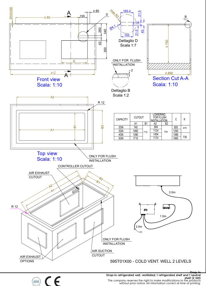
Drop-in Drop-in refrigerated well, ventilated, 1 refrigerated shelf and 1 neutral shelf (2 GN) The company reserves the right to make modifications to the products without prior notice. All information correct at time of printing.
